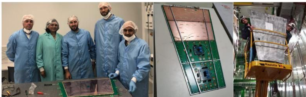
Fig. 4: Left: Preparation towards the second station of GEMs in CMS- single module. Middle: A complete GE21 Detector. Right: Installation exercise for GE21.
