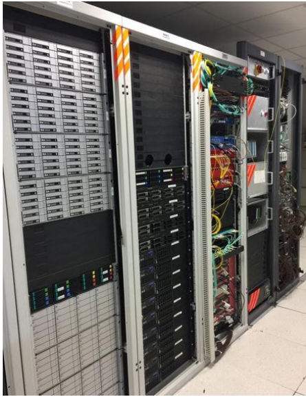
Figure 2: Racks hosting the ProtoDUNE-SP Trigger and Data Acquisition system. The system is connected to the on-detector electronics through up to 300 optical fibers. A local temporary storage of 700 TByte is also available.
