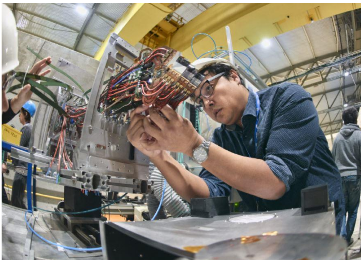
Prototype vertex locator (VELO) pixel modules were developed and tested in a beam in the North Area last year ahead of the upgrade (Image: Julien Marius Ordan/CERN).
