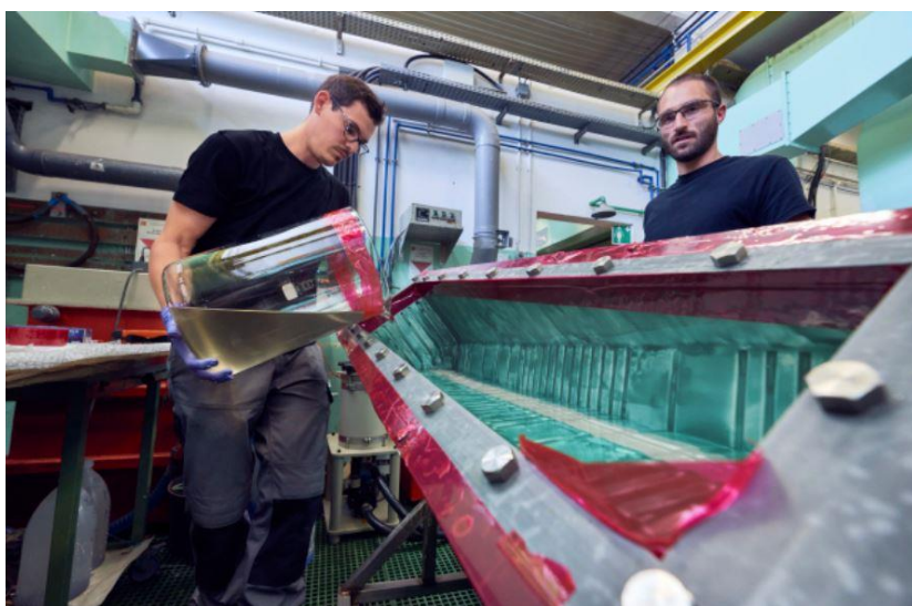
Pierre Maurin (left) and Florent pours an etching solution into a prototype RF box in order to remove another 100 micro-meter of aluminium. The green paint protects parts of the box that should not be thinned further. (Image: Maximilien Brice /CERN).
