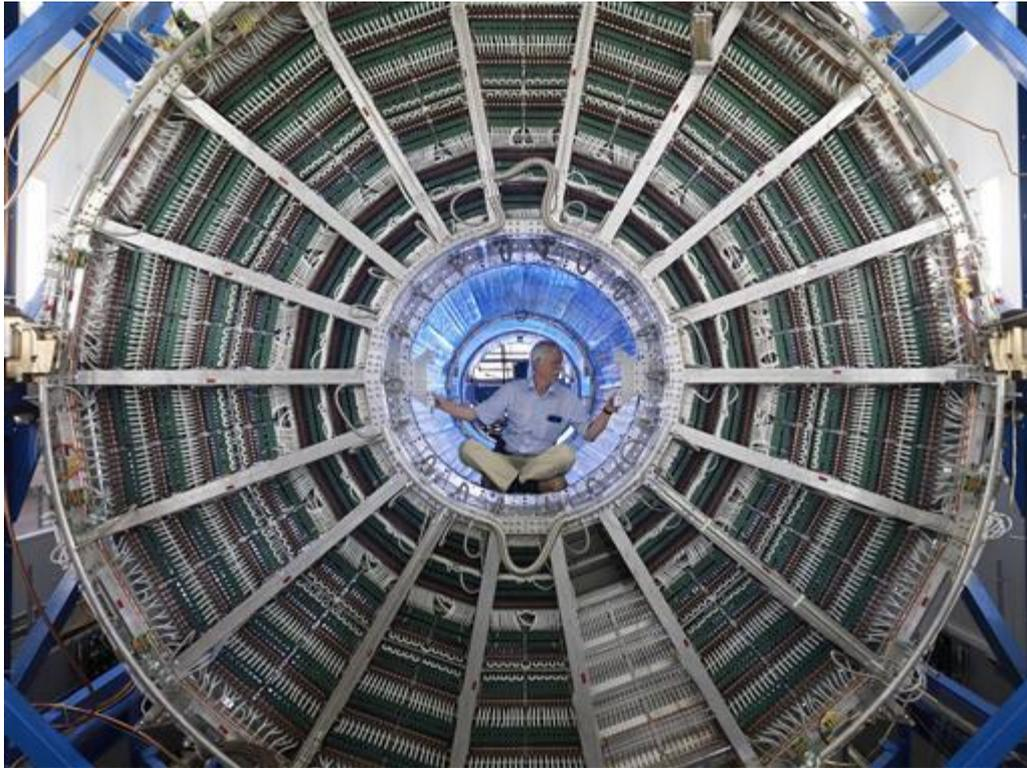
**ALICE Time Projection Chamber (TPC), the largest in the world at nearly 100 cubic metres, will also be upgraded during LS2.**
