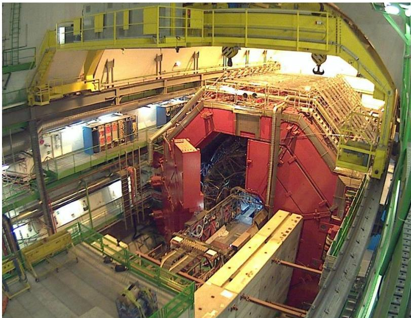
**The ALICE solenoid re-opens its door as the collaboration prepares for the detector upgrade planned for LS2.**
