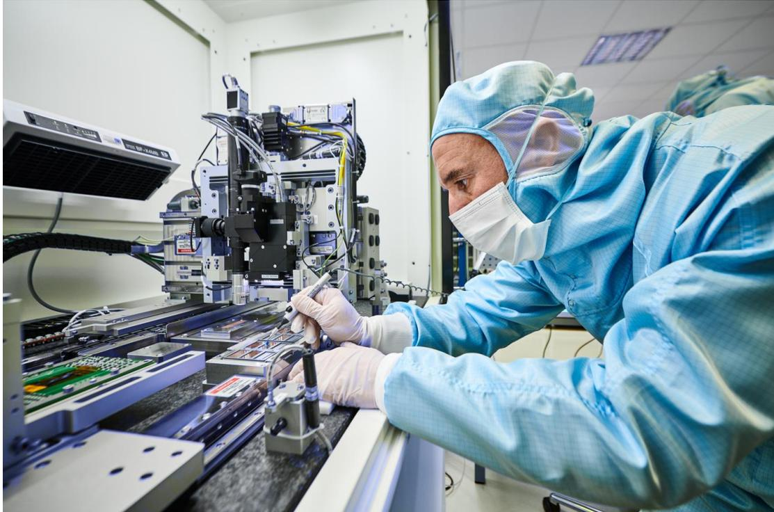
**Mounting of a module of the New Inner Tracking System (ITS) of ALICE, which will be installed in the heart of the experiment in 2020**
