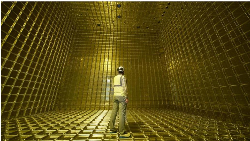
*Figure 1: Inside of the ProtoDUNE detector cryostat.*
