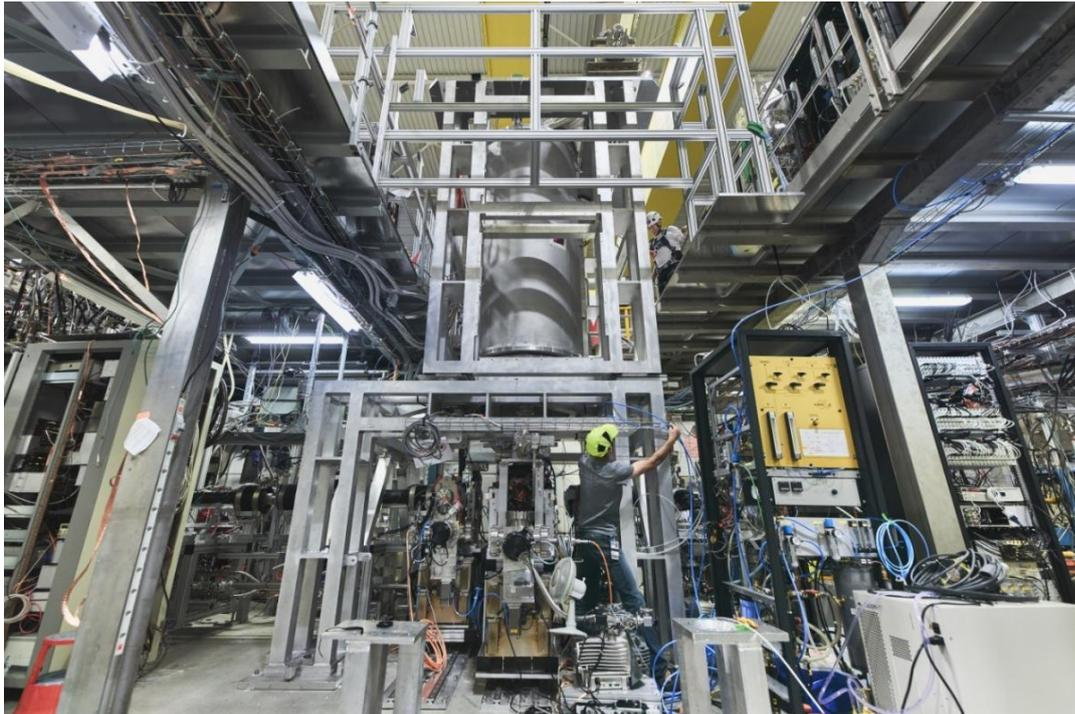
The ALPHA-2 device has seen a string of successes in recent years, the latest being the observation of laser spectra of the 1S-2S and 1S-2P transitions in antihydrogen. The former led to the most accurate measurement on antimatter ever achieved with an accuracy of 12 significant digits in the transition frequency, and the latter paves the way to laser-cooling amongst other things.
