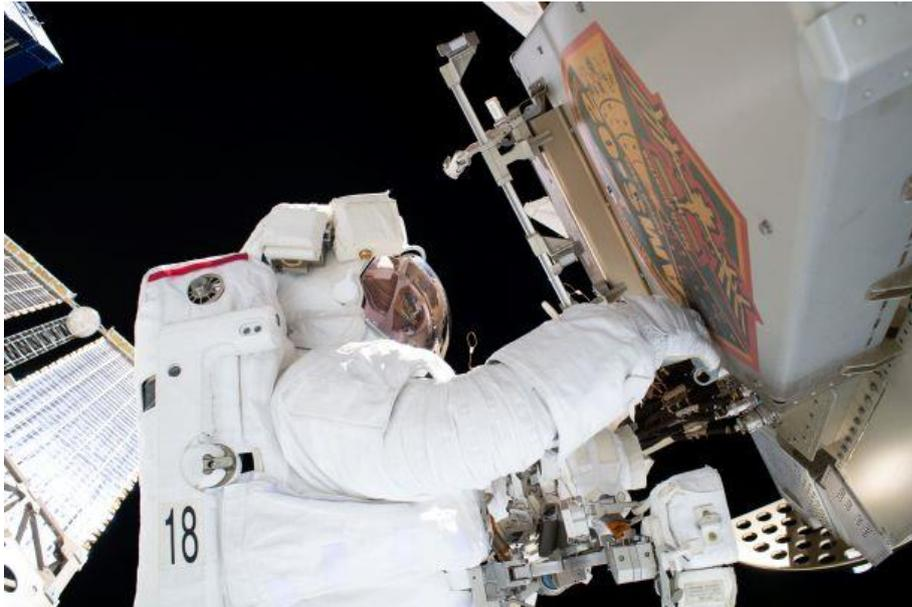
**Figure 1: Preparing to remove the AMS-02 detector debris shield and gain access to the main working site.**
