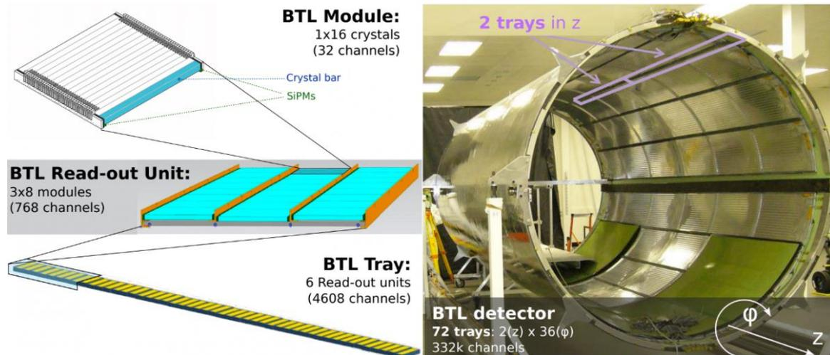
**Overview of the BTL showing the hierarchical arrangement of the various components, bars, modules, Readout Units, and trays, inside the Tracker support tube.**
