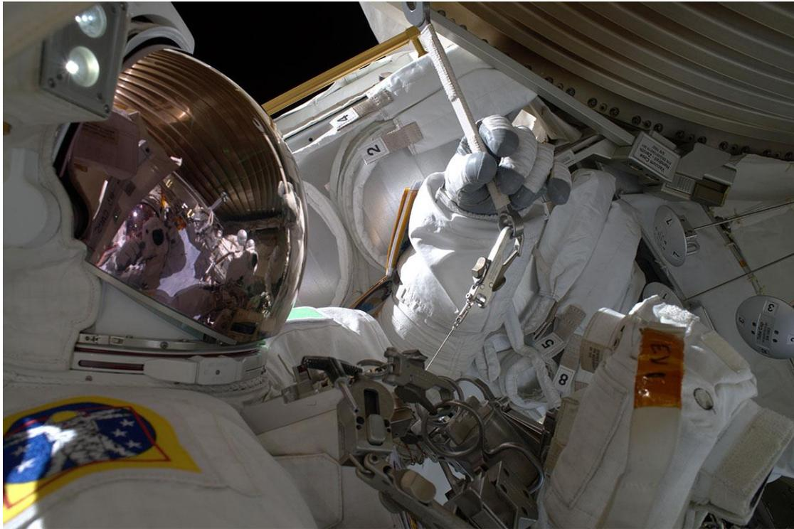
**Figure 3. The long process to swage (connect) the tubes is completed using a specially designed 7/8” wrench. (via @Luca Parmitano Twitter account, Credit: NASA).**
