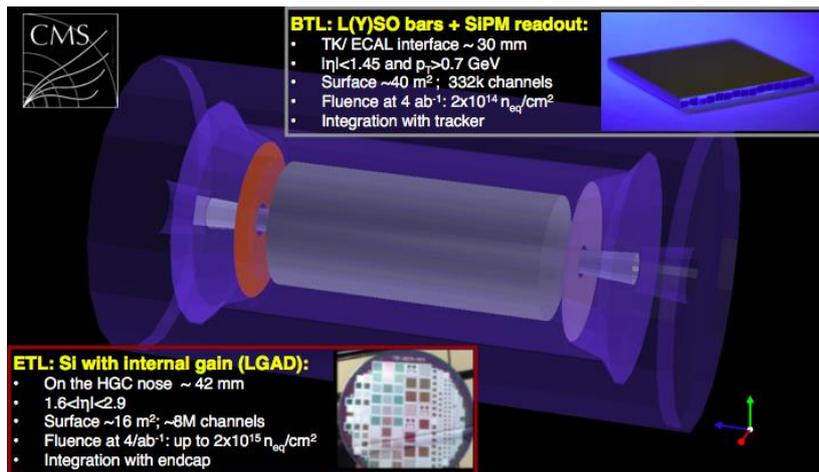
**A schematic view of the GEANT geometry of the timing layers implemented in the CMS software for simulation studies comprising a barrel layer (grey cylinder), at the interface between the tracker and the ECAL, and two silicon endcap (orange and light violet discs) timing layers in front of the endcap calorimeter.**
