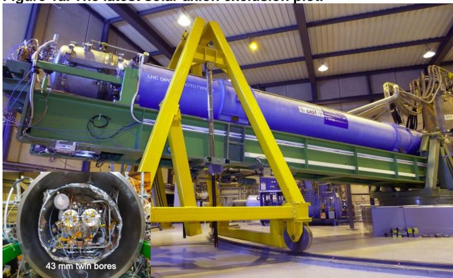
Figure 1b: CAST experiment and close up photo of the twin bores of the CAST magnet where the RADES and CAST-CAPP RF cavities are installed.
