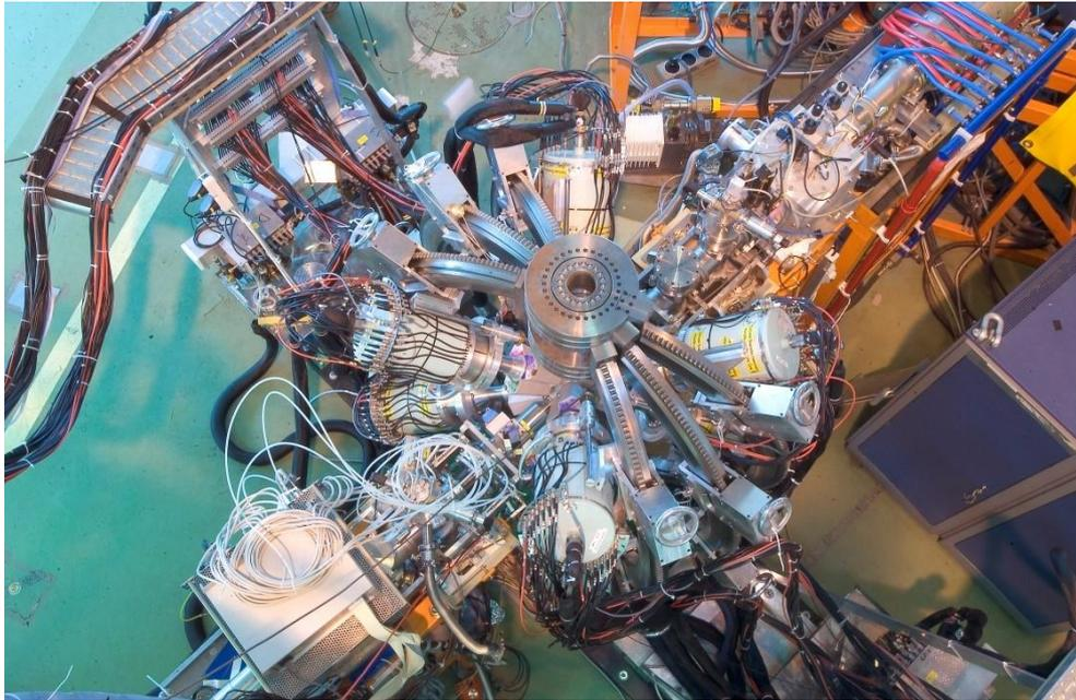
**Figure 1: The Miniball spectrometer in the ISOLDE experimental hall.**
