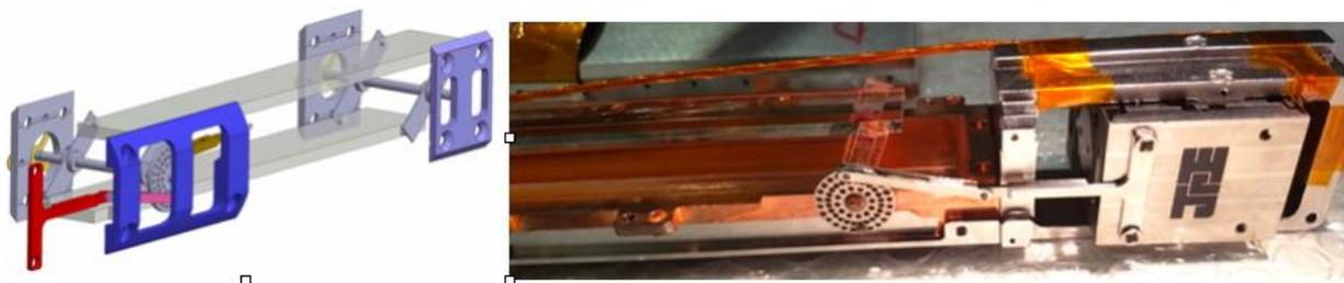
**Figure 2: The tuning mechanism of CAST-CAPP detector (left) and the stepper motor providing the movement through the locomotive mechanism (right).**
