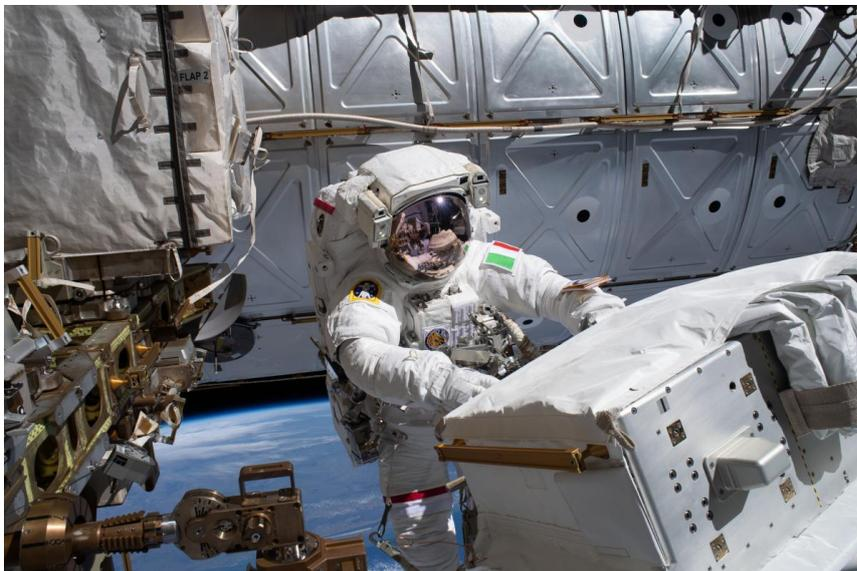
**Figure 2. During a spacewalk earlier this month, Luka Parmitano carried out of the ISS the box with the new pumps to be installed in AMS-02 (Credit: NASA).**
