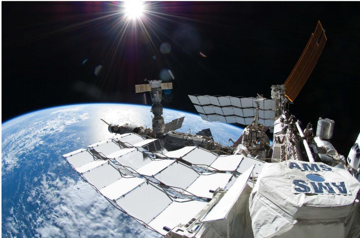
The detector consists of a series of components that record the identity, trajectory and momentum of subatomic particles zipping around the cosmos. Just as visible light allows astronomers to study distant stars and galaxies, these particles—cosmic rays—enable physicists to study the far reaches of the universe. AMS-02 also allows physicists to search for evidence of dark matter, an elusive material that has so far been observed only through its gravitational pull on visible matter.
