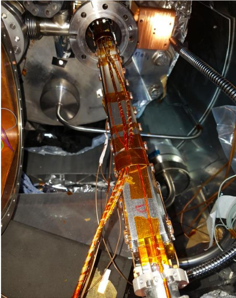
**Figure 1c. Installation of CAST-CAPP RF cavities on one of the two bores of CAST magnet**
